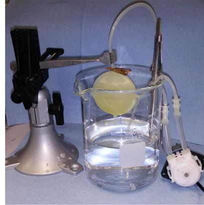
Fig. 3. internal support material removal system
