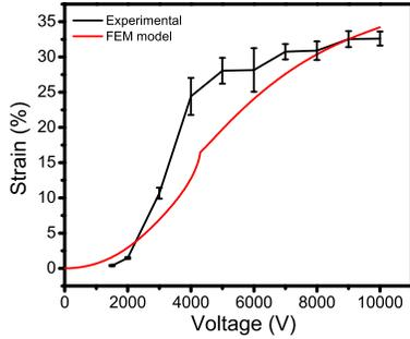
Fig. 4. Strain voltage curves of FEM model and experimental results of actuator fabricated in Tangoblackplus
