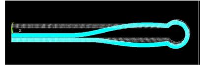
Fig. 2. Predicted Deformation of a donut type actuator with 0.625 mm wall thickness at 10KV
