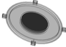
Fig. 1. CAD model of actuator with black regions denoting a CNT coating
