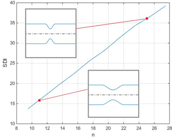
Fig. 4. SDI for beam B1 of Fig. 2 vs.  $n$ . Two different geometries are shown in the insets: for  $n = 11$ , it is  $\text{SDI} = 15.9$ ; for  $n = 25$ , it is  $\text{SDI} = 36.6$ .
