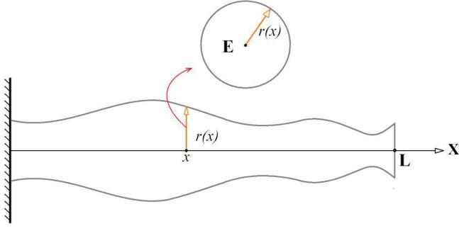
Fig. 1. Cantilever beam with variable cross section of radius  $r(x)$  and variable Young's modulus  $E(x)$
