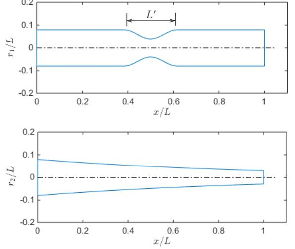
Fig. 2. Side view of beams B1 (top) for  $n = 8.5$  and B2 (bottom).
