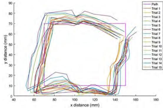
Fig. 6: Open-loop soft robot path tracking
