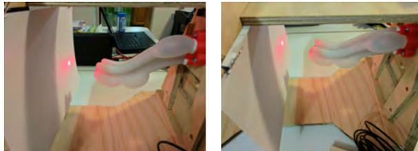
Fig. 1: Soft robot with no rigid sections designed using a complementary approach that eases subsequent tip trajectory tracking.
