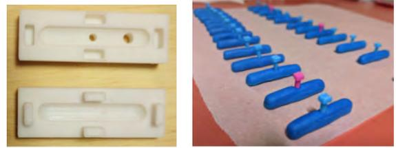
Fig. 2: Moulds (*left*) and sacrificial chambers from them (*right*) to support multiple air pockets in a single casting).
