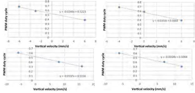
Fig. 5: Vertical velocity scaling values (for the same the 4 of the 12 valves shown in Fig. 4)
