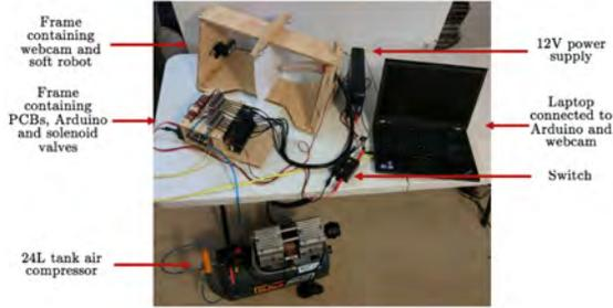
Fig. 3: Assembled soft robot testing system
