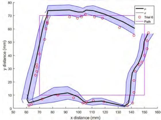
Fig. 7: Soft robot overall tracking (path mean [solid black] and standard deviation [shaded])
