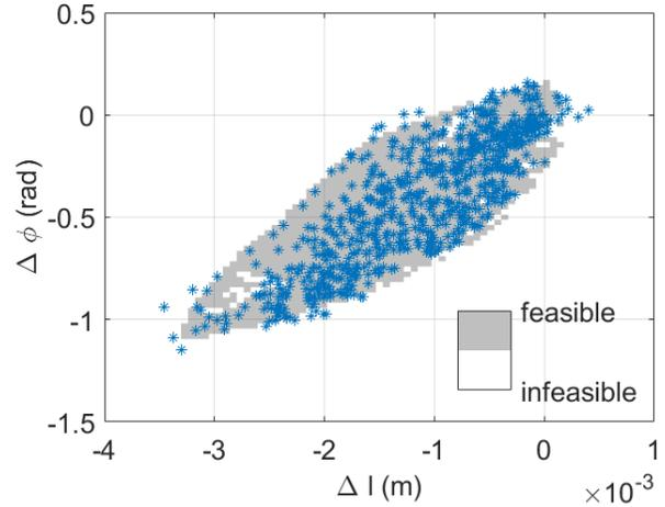
Fig. 2. The workspace calculated by the method described in section II in grey, overlaid with the set of achievable points found by sweeping over the entire range of admissible pressures and measuring end effector positions.
