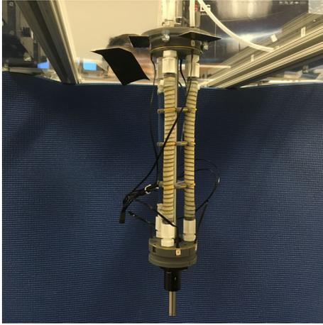
Fig. 1. System comprised of a parallel combination of three FREE actuators as described in section III. The end effector is constrained to 2DOF motion by a central rod and linear/rotary bearing.
