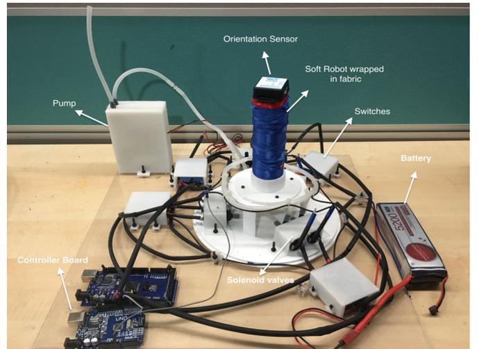
Fig. 6: Experimental Platform developed to demonstrate the effectiveness of the proposed oscillation damping method.
