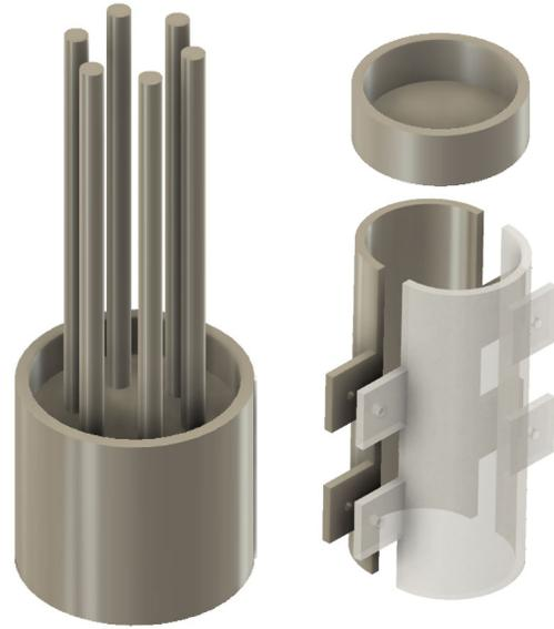
Fig. 3: 3D drawing of the molds used to cast the 6-chambered parallel soft robot. Left: base of the mold, top right: cap of the mold, and bottom right: the wall to be inserted in mold base.
