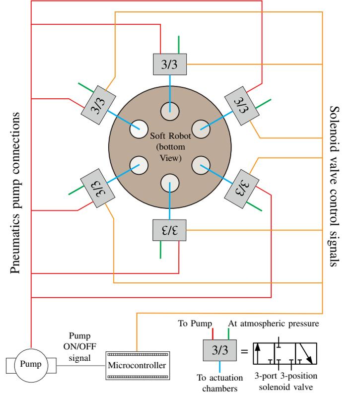
Fig. 4: Schematic diagram of the actuation mechanism developed for the parallel soft robot used in our experiments.
