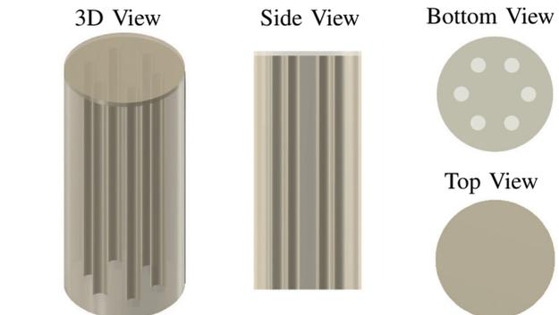
Fig. 1: 3D model of the 6-chambered parallel soft robot. Left: 3D view of the model, top right: side view, and bottom right: bottom view of the soft robot model.
