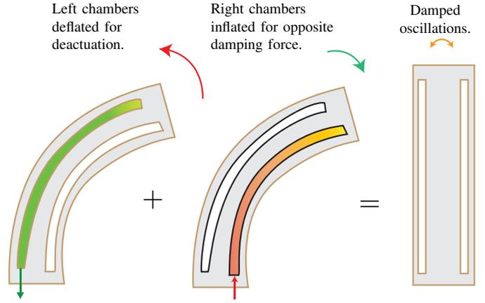
Fig. 5: 2D illustration of the active oscillation damping mechanism during deactuation. The damping force is created by simultaneous deactuation of left chamber and actuation of right chamber.
