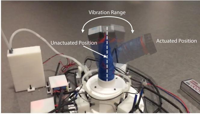
Fig. 2: The oscillations produced in soft robot on deactuation.
