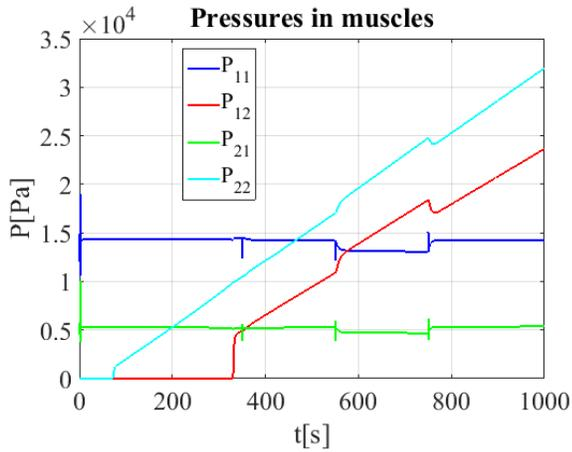
Fig. 6: Inflated pressures in soft robot arm antagonistic pairs of actuators
