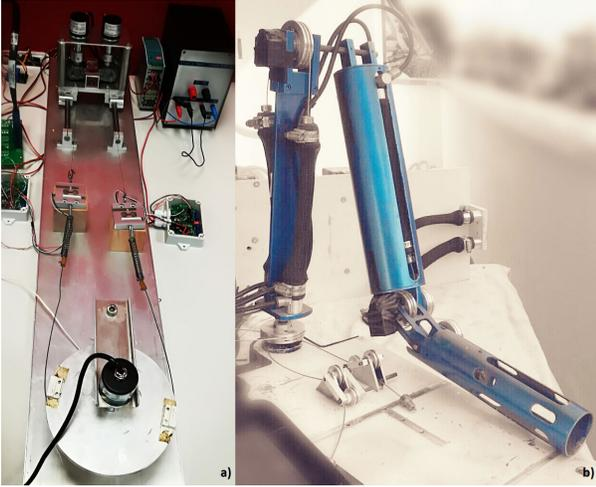
Fig. 1: Laboratory setups for antagonistic compliant actuators: (a) Actuator driven by electrical drives and nonlinear extension springs at University of Belgrade (b) Actuator driven by pneumatic McKibben drives at University of Palermo at courtesy of University of Pisa;
