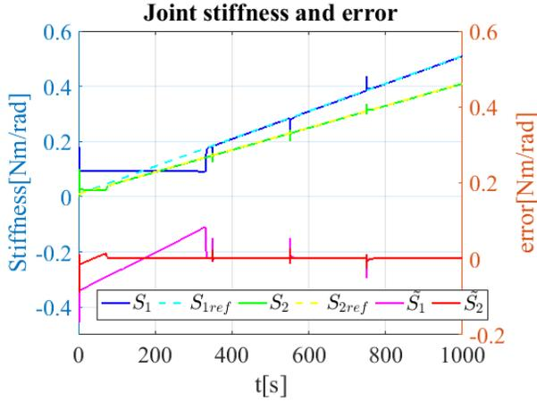
Fig. 5: Trajectory tracking simulation of soft robot arm stiffness
