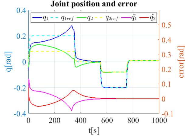
Fig. 4: Trajectory tracking simulation of soft robot arm joint position
