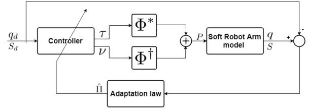
Fig. 3: The diagram of adaptive control
