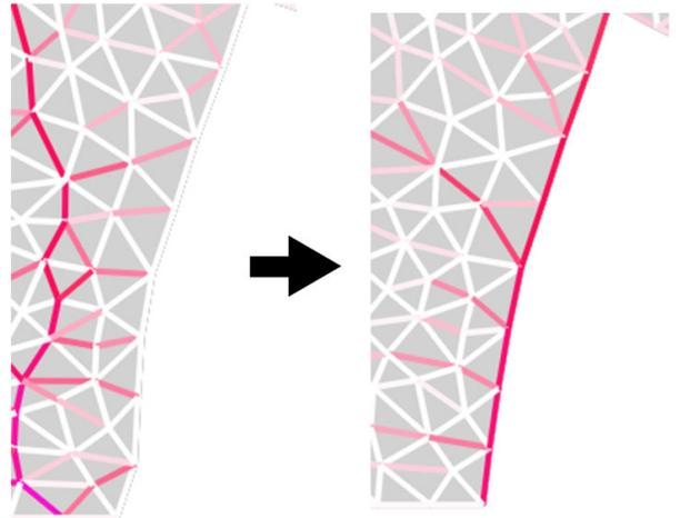
Fig. 6. Our objective is highly non-convex, especially in the presence of the sparsity regularization.  $\mathcal{O}_{\text{continuity}}$  can be used to explore potentially better local minima. In this example, a messy activation pattern can be seen. Enabling  $\mathcal{O}_{\text{continuity}}$  allows the solver to converge to a cheaper and smoother solution.
