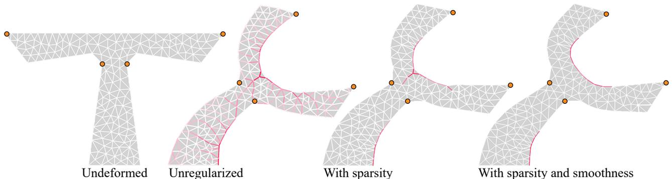
Fig. 2. Regularizing the tension in the T shape. (From left to right) The T shape in its undeformed state and the target deformation without regularization. Red segments are fibres that are tensioned. Without any regularization the activation pattern presents itself to be very dense. Applying an  $L_0$  regularizer causes significant sparsification of activation. We further apply a smoothing regularizer to encourage continuous final tendons with the result being depicted on the right.
