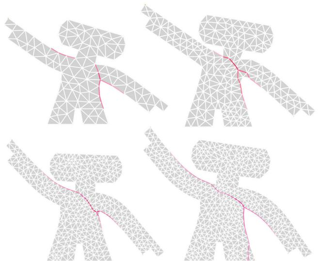
Fig. 3. Robot mesh with target pose and corresponding activation pattern. Both sparsity and smoothness regularization have been used. The calculation has been done on meshes with four different triangulation densities. For comparison see [3].
