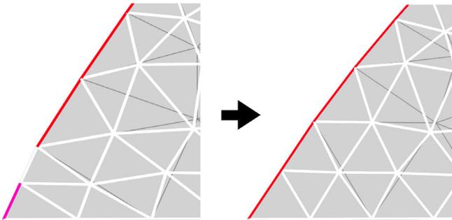
Fig. 4. The smoothness regularizer closes gaps in active fibre strands. In this case,  $\mathcal{O}_{\text{continuity}}$  drives the activation gap up in tension to enforce equitension in the chain.
