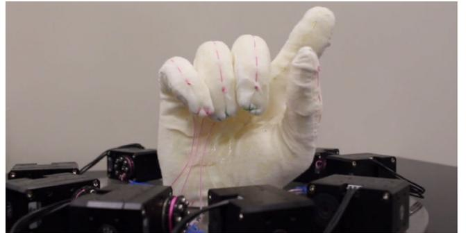
Fig. 1. A soft robotic hand with naive tendon routing. A more clever actuation layout could have likely achieved this pose with fewer tendons
